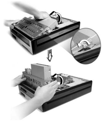
4 Pull out the drive rails that hold the hard disk to the housing. Set the drive rails aside.
